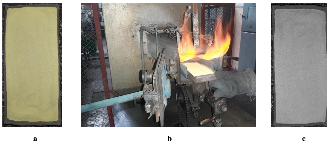
Figure 1. \text{WO}_3 powder loaded into the boat (a), process of loading the boat into the furnace (b) and W powder coming out of the furnace (c)
